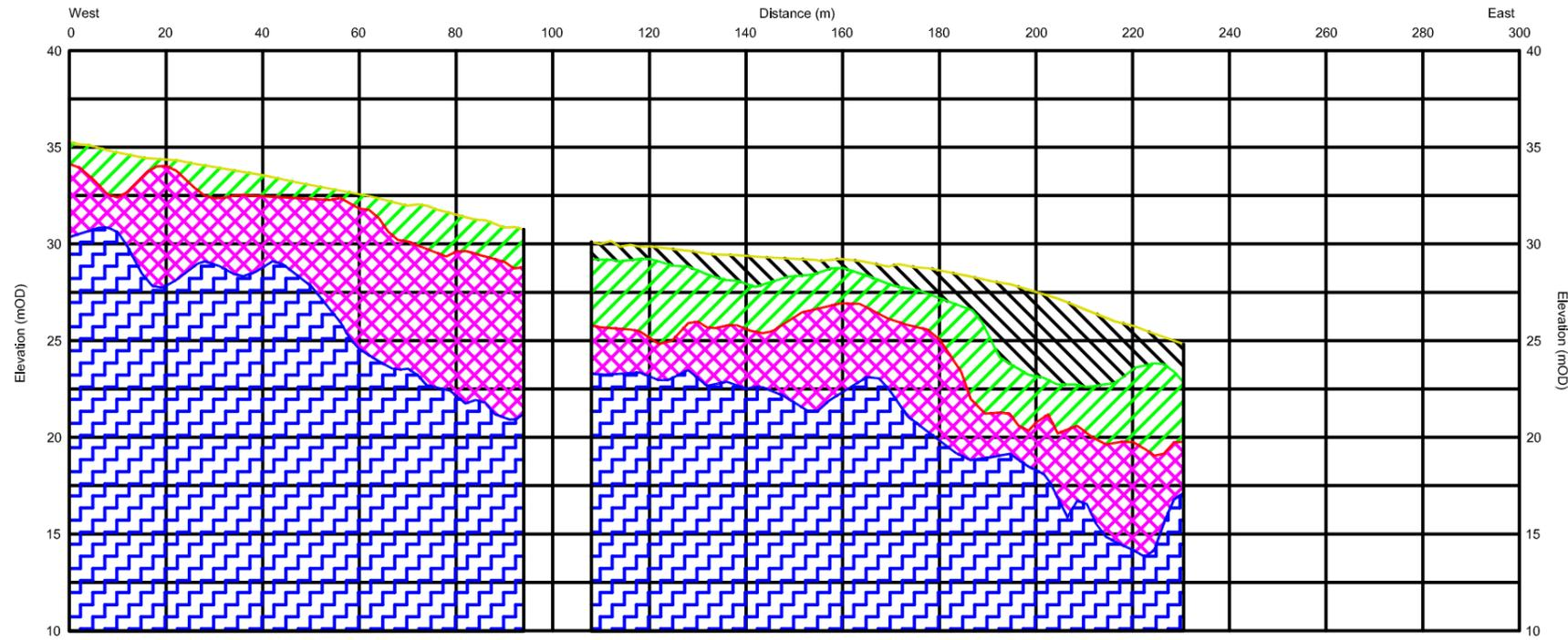
Seismic Refraction Line 4 (S32 - S27) Interpretation
