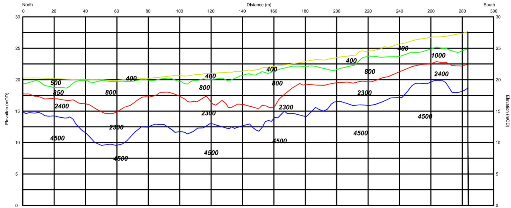
Seismic Refraction Line 5 (S26 - S20) Model
