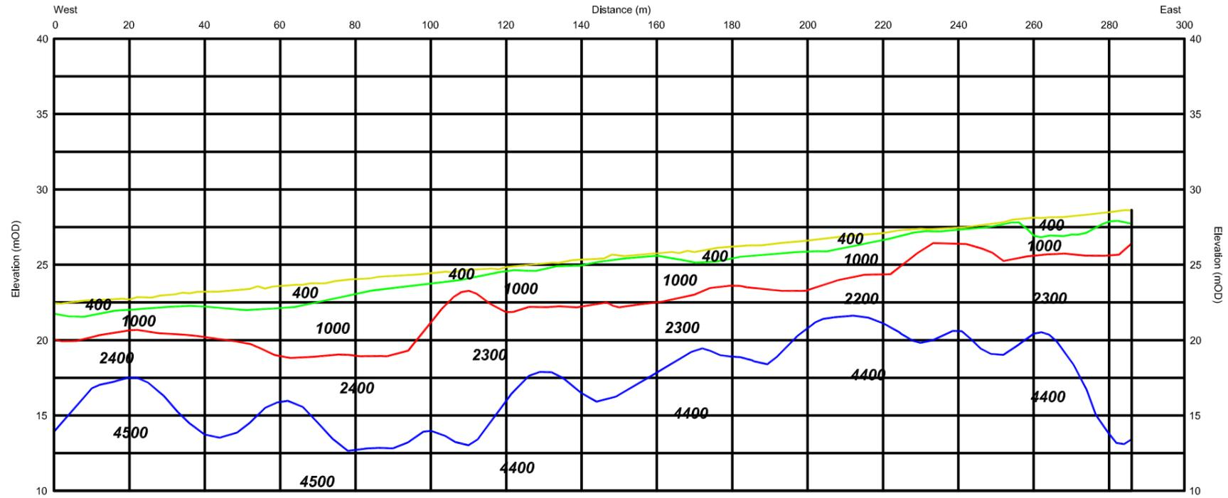
Seismic Refraction Line 2 (S9 - S6) Model
