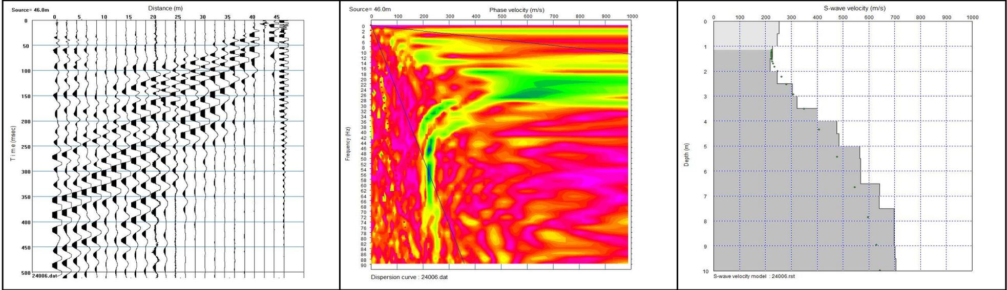
MASW Results from Line 6, Profile 1, Shot 5, Traces 13-24. From left to right images show the seismic shot record, the dispersion curve and the shear wave velocity - versus depth model.
