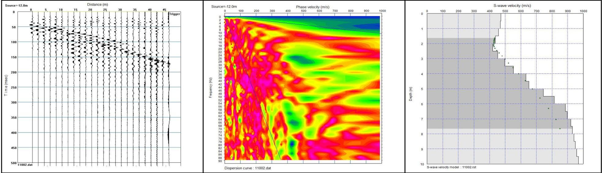
MASW Results from Line 8, Profile 16, Shot 6. From left to right images show the seismic shot record, the dispersion curve and the shear wave velocity - versus depth model.
