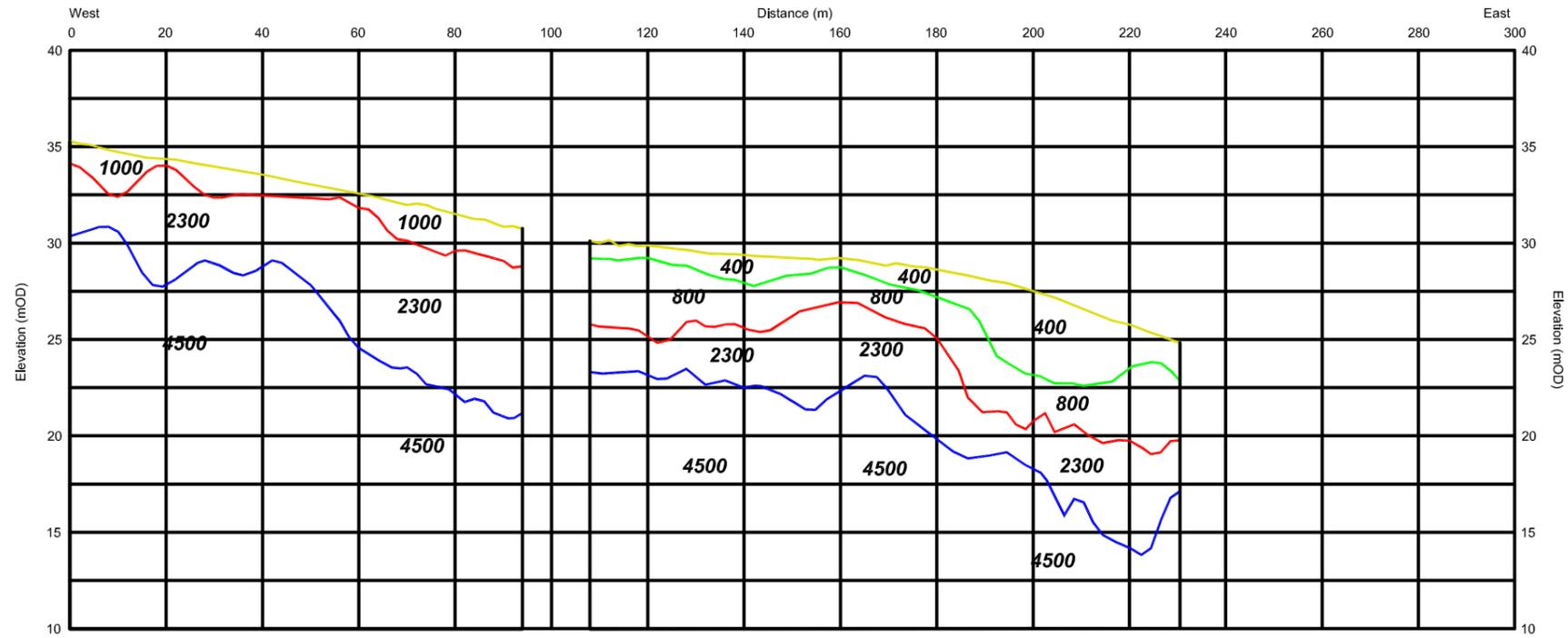
Seismic Refraction Line 4 (S32 - S27) Model
