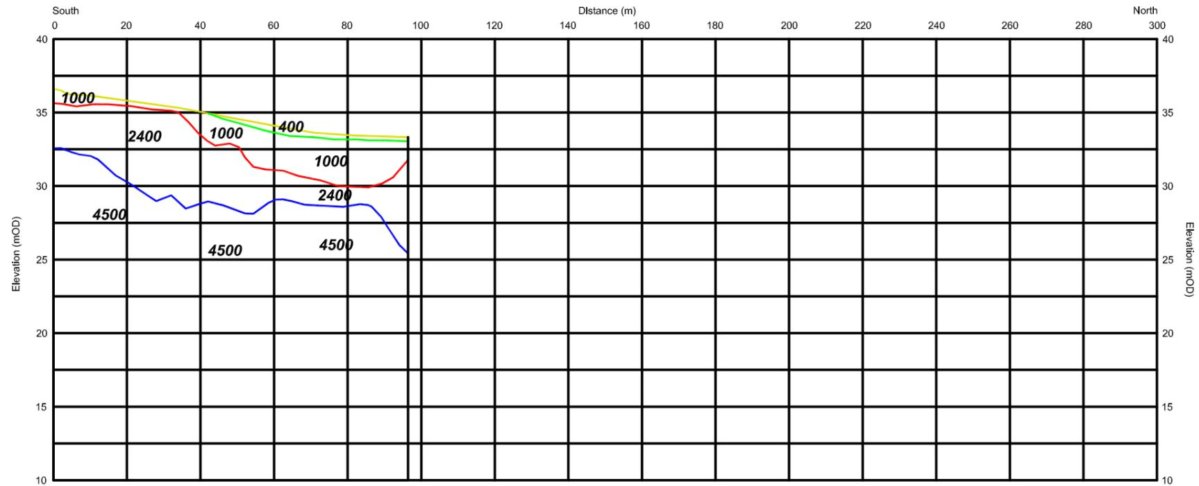
Seismic Refraction Line 8 (S15 - S17) Model
